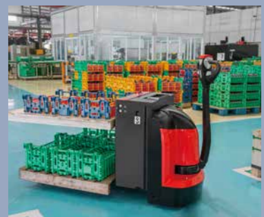
The support arm lift capacity is 2000 kg while the mast lift capacity is 800 kg
