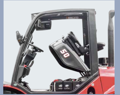
The easy-to-open hook provides quick access to the engine compartment
