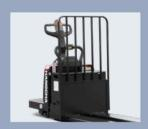
The load backrest is secured with high-strength bolts, which can protect the operator effectively
