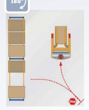
In the mode of 180-degree steering, the truck must be reversed until it stops completely, and the direction must be switched before the truck can travel forward, with lower efficiency.
