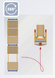
In the mode of 360-degree steering, when steering exceeds 270 degree, the reverse is switched to forward director, no reversing is required, and the truck is switched to advance automatically, no parking is required, with higher efficiency.
