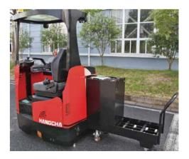
Standard configuration: Battery side roll-out + trolley(optional)
